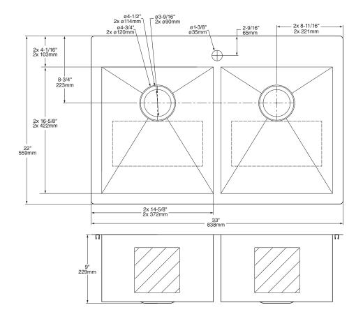
NOTES: \* DIMENSIONS SHOWN FOR LOCATION OF SUPPLIED AND "P" TRAP ARE SUGGESTED. FITTINGS NOT INCLUDED WITH FIXTURE AND MUST BE ORDERED SEPARATELY. SEALING COMPOUND SUPPLIED BY OTHERS.
